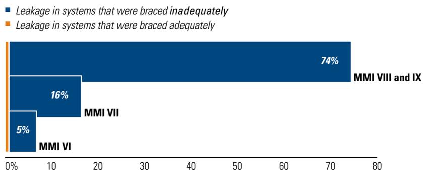
As illustrated here, the Northridge earthquake demonstrated that sprinkler systems can fail at earthquake intensity levels above MMI VI when not braced as recommended by FM Global.
